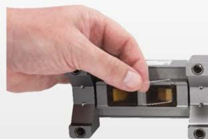
Placing the coupling pads before installation on the transducer surface
