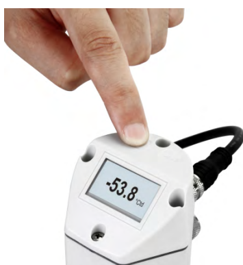
Alarm adjustment at dew point sensor
